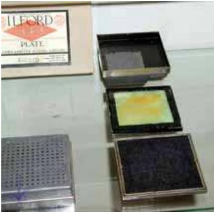
*Fig. 1 The first scintillation camera with collimator developed by Sven Johansson and Bengt Skanse. A photographic film was placed directly on the sodium iodide crystal.*
